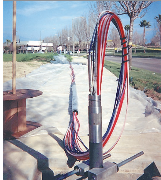
Contaminant investigation at a U.S. Air Force Base. Waterloo Systems installed to 700 ft. in overburden using screened and cased wells. Up to 6 zones per hole with dedicated pumps and transducers.
