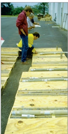
Using core logs to identify placement of Ports and Packers (left). Multi-Purge Manifold with transducers and dedicated pumps for four zone monitoring (right).
