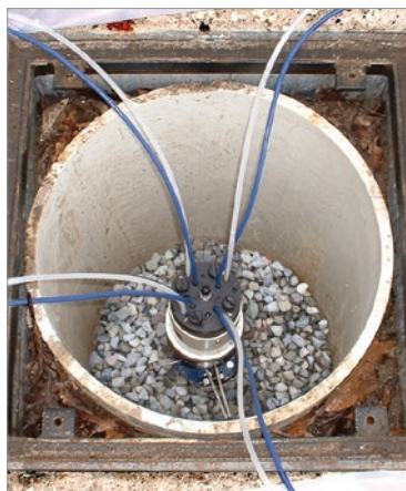
Using core logs to identify placement of Ports and Packers (left). Multi-Purge Manifold with transducers and dedicated pumps for four zone monitoring (right).
