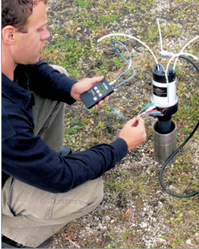
Collecting a sample from a dedicated DVP and taking pressure measurements with Model 404 Geokon Vibrating Wire Readout.
