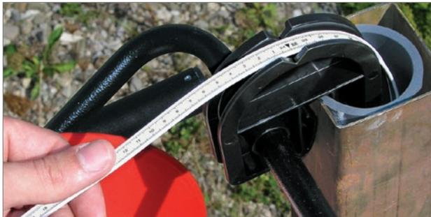
A Tape Guide allows depth measurements to be read at the marked position on the Tape Guide, to give reliable, repeatable, accurate depth measurements when profiling a well. The Tape Guide protects the tape from damage on rough edges of well casing.
